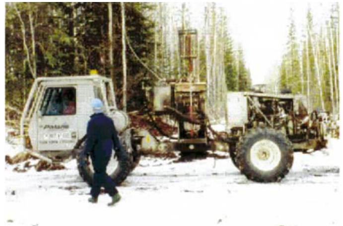
Figure 5: Accelerated Weight Drop system
